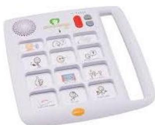
A portable dedicated speech generating device that features 12-message locations and 12-minutes of record time. Simply switching between the five available recording levels provides up to 48-messages. Includes built-in carrying handle.
