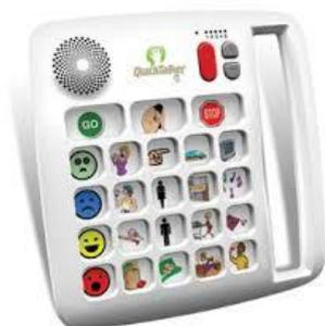
A portable dedicated speech generating device that features 23-message locations and 20-minutes of record time. Simply switching between the five available recording levels provides up to 103-messages. Includes built-in carrying handle. Requires 4 x AA batteries (not included).
