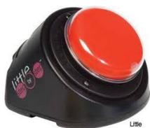
Record any series of messages into the LITTLE Step by Step Communicator. Press its activation surface once to hear the first message. Press it again to hear the next message in the sequence, and so on. Two full minutes of recording time. LITTLE Step by Step features an angled base and 6.25 cm activation surface. Requires 9V battery (not included).
