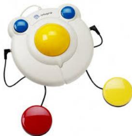
The BIGTrack has a 7.5cm trackball which makes it the largest trackball available. The large ball requires less fine motor control than a standard trackball and it is ruggedly built. It has a left and a right mouse click button located behind the trackball to avoid unwanted mouse clicks.
