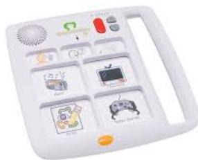
A portable dedicated speech generating device that features 7-message locations and 6-minutes of record time. Simply switching between the five available recording levels provides up to 23-messages. Includes built-in carrying handle.
