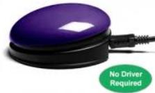
USB Switch is a low profile 75mm switch with a built-in USB interface. The switch can be configured to operate as a wide variety of keyboard, mouse and gamepad functions and is programmed via an integral LED display. This switch also allows a number of additional features to be configured to help compensate for various motor deficits and neuromuscular conditions, including Acceptance Delay, Ignore Repeats, Maximum Press Time etc.
