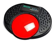
A versatile AAC device with 5 adaptive levels and 8 playback modes, offering 8 minutes of recording time.
